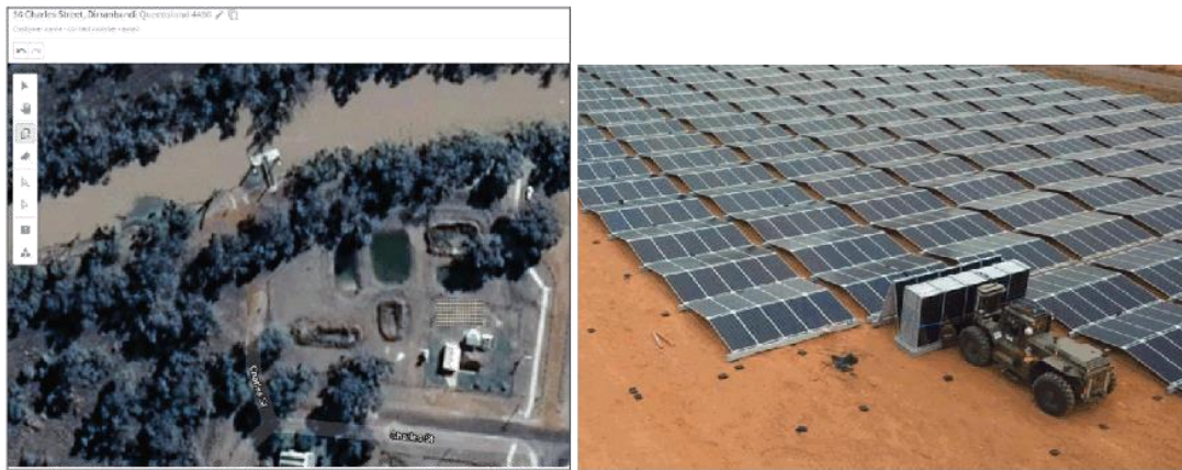
Figure 24: WTP showing east-west array within perimeter fence, and a sample of this array type on the right (source: 5B.com.au).
