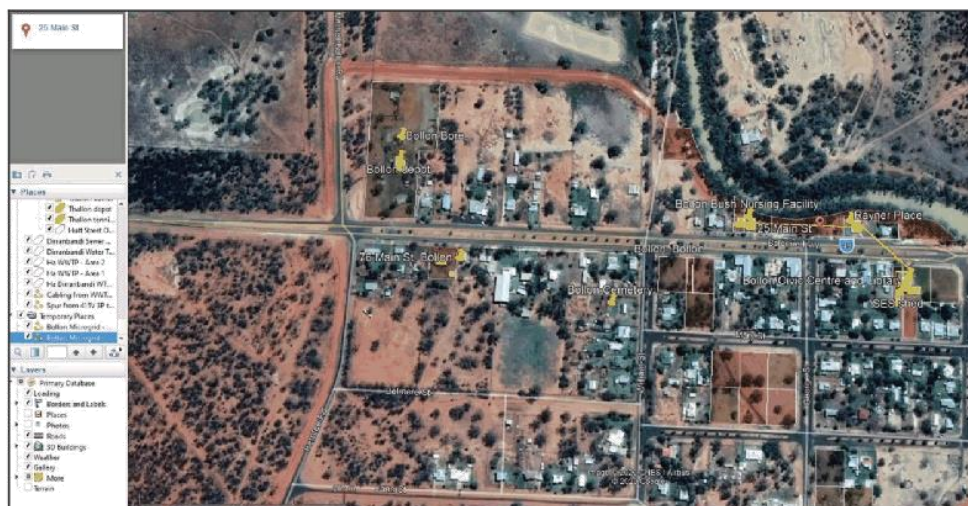
Figure 75: Layout of Bollon microgrid with yellow line showing one option for power reticulation
