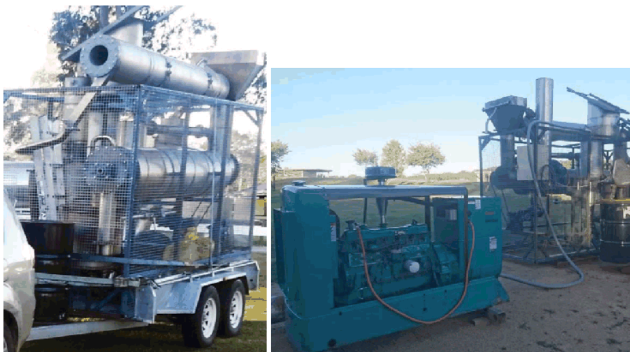
Figure 89: Portable ID gasifier showing towing capability
