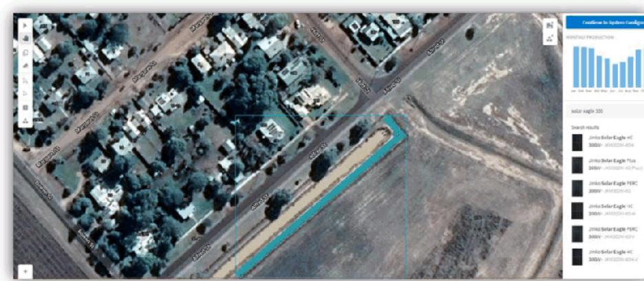
Figure 9: Example footprint of ground mounted reticulated power from 157 kW array
