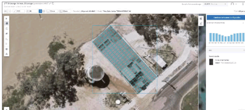
Figure 8: Example footprint of 93.6 kW array at Hutt St
