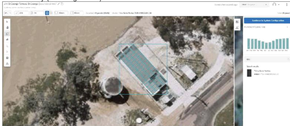
Figure 7: Example footprint of 40 kW array at Hutt St
