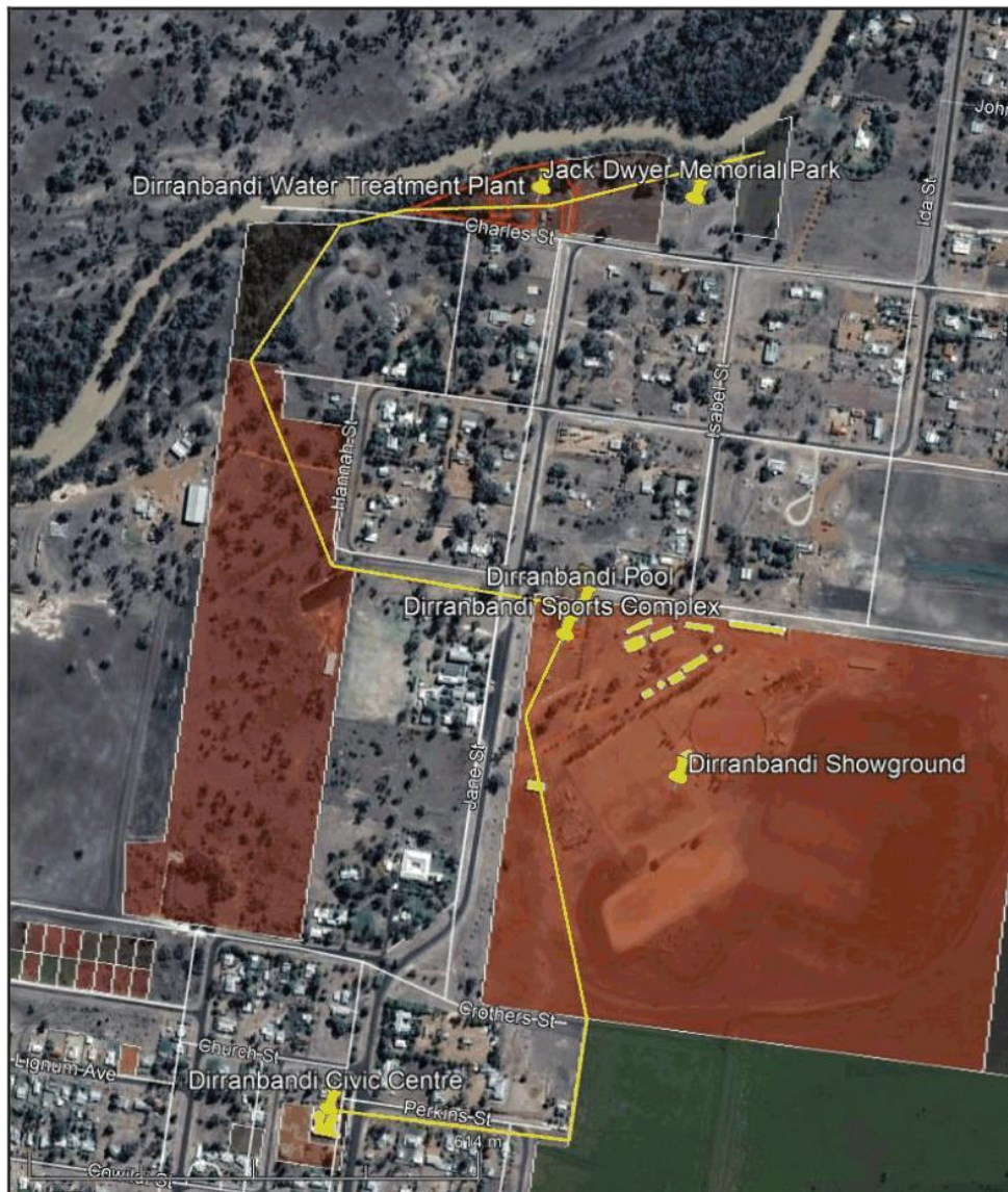
Figure 74: Location of Dirranbandi microgrid with the yellow line showing one option for power reticulation
